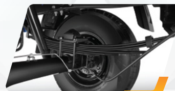
Leaf Springs Front: Parabolic for Superior Comfort Rear: Semi Elliptical for Carrying More Load
